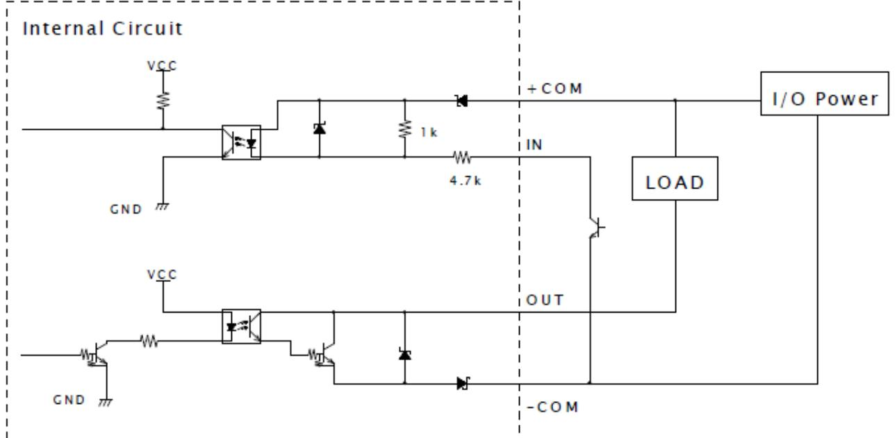
Connect both +COM and -COM to I/O Power.
