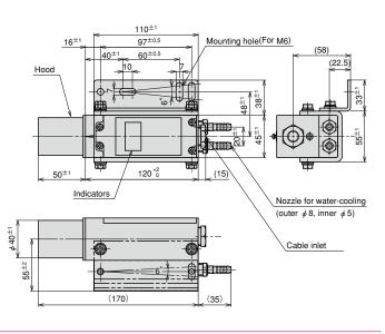
Through-beam Type Detector (CMD)
