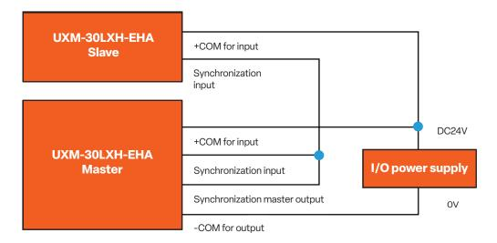
Synchronization master output of the master's sensor is connected to the synchronization input of the master itself and to the synchronization input of all slave sensors.
