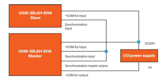
Synchronization output of the master sensor is connected to the synchronization input of the master itself and to the synchronization input of all slave sensors.
