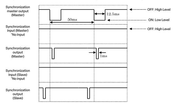
When synchronization master output of the master is connected to the synchronization input of the slave Falling edge of the synchronization master output signal and falling edge of the synchronization output signal which are connected to synchronization input of the slave are synchronized. Based on the phase setting performed by means of the application program, the motor rotation of the slave is shifted by the setting amount. Error of phase setting shall be within <u>+</u> 1 ms.
