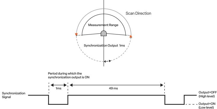
During malfunction, synchronization output is OFF
