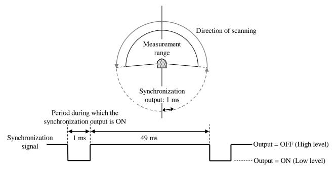
During malfunction, synchronization output is OFF.
