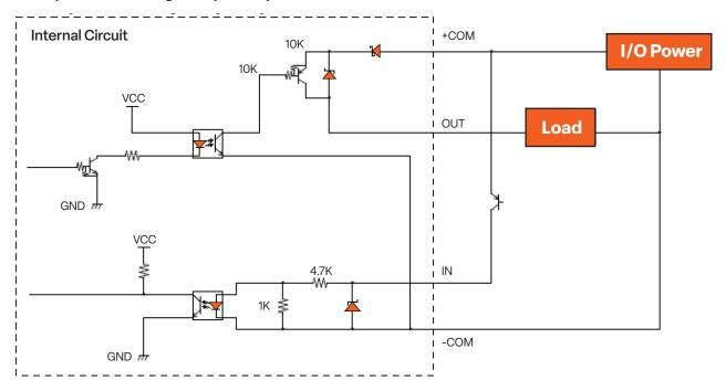
Connect both +COM and -COM to I/O Power.
