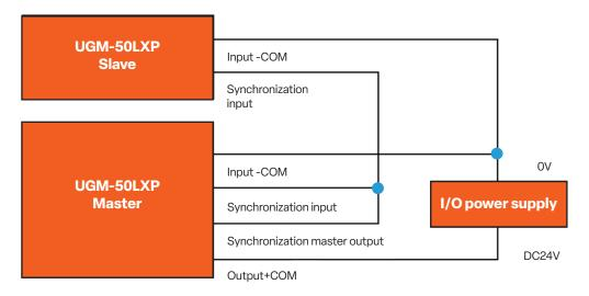
As shown in the figure above, it is possible to synchronize the motor rotation of the slave with the motor rotation of the master according to the shifted scanning time of each slave sensor by setting phases of each slave sensor.
