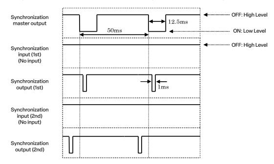
When synchronization master output of the master is connected to the synchronization input of the slave Falling edge of the synchronization master output signal and falling edge of the synchronization output signal which are connected to synchronization input of the slave are synchronized.
