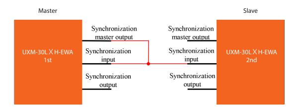
Synchronization master output of the master's sensor is connected to the synchronization input of the master itself and to the synchronization input of all slave sensors.
