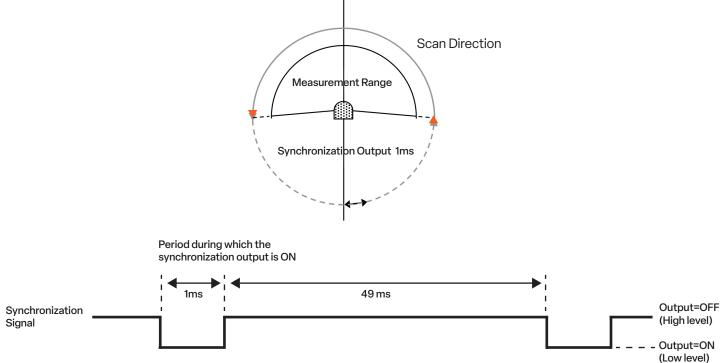
During malfunction, synchronization output is OFF
