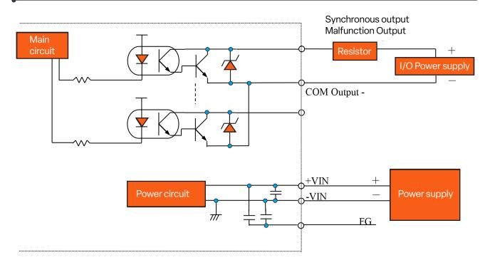
Note: Mounting plate is used as frame ground (FG). Mount the sensor on a stable structure..
