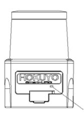
Power supply display (Blinks during start up and malfunction state)
