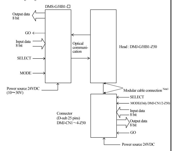
Note 1) Make sure not to use the combination with DMJ-G/HB1-Z50 and DMJ-CN1~4, and DMJ-G/HB1 and DMJ-CN11~4-Z50.
